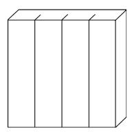
**Single Cut Grooves (one surface):** Saw cuts are made on one surface of the core to allow flexibility with minimal interference with resin absorption.
