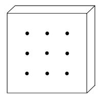
**Perforations:** Holes are pierced through the core material with a diameter of 2mm and a standard perforation pattern of 2" x 2" or 1" x 1".
