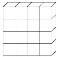
**Contour Cut:** Core is slit all the way through and backed with a fiberglass scrim. This configuration provides the most flexibility.
