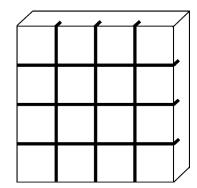
**Grooving:** Superficial saw cuts are made 2.5mm deep and 1.5mm wide with a standard spacing pattern of 30mm x 30mm.
