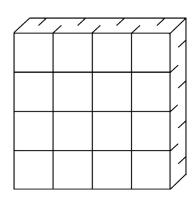
Cross Cut Grooves (both surfaces): Saw cuts are made on both surfaces in both directions to allow greater directional flexibility and more resin flow.
